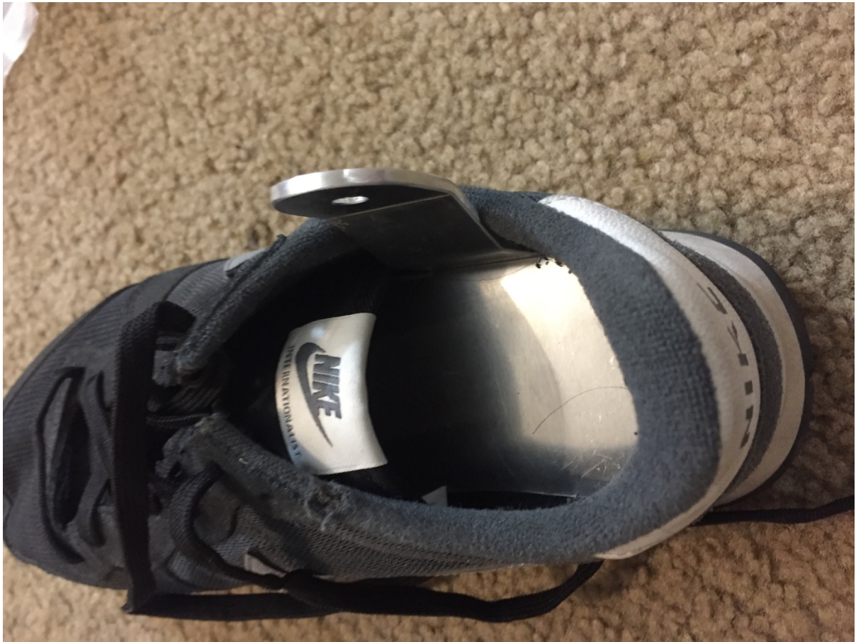
Figure 4 Inserting Footplate inside a Shoe
