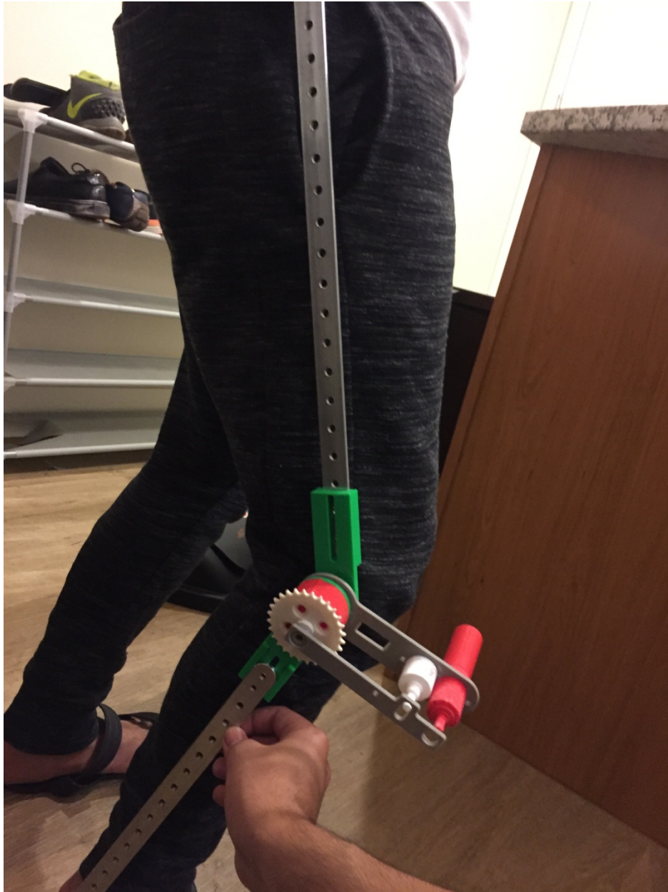
Figure 6 Attaching the Frames to the Motor
